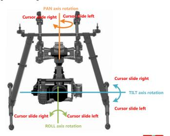
MODE: Toggle the 3-position switch, the corresponding slider of cursor will turn red
