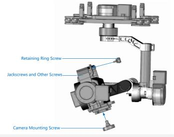
**Step4:** Mount the camera into the gimbal and tighten the camera mounting screw.
