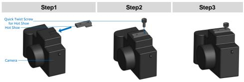
**Step1:** Insert the hot shoe into the camera.
