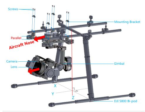
**Step7:** Install gimbal to a bi-pod with mounting bracket; tighten up screws (2.5\*8 Head-cup screwx8) with appropriate screw glue.
