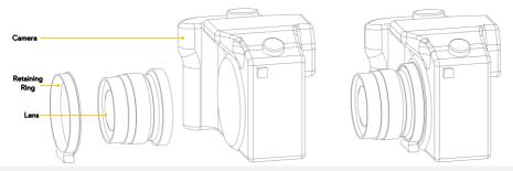
stepl: Mount the lens onto the camera first, and then put the retaining ring through lens until it is fixed.
