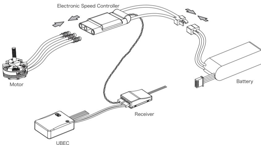
This is an extremely powerful brushless motor system. We strongly recommend removing your propellers for your own safety and the safety of those around you before performing calibration and programming functions with this system.
