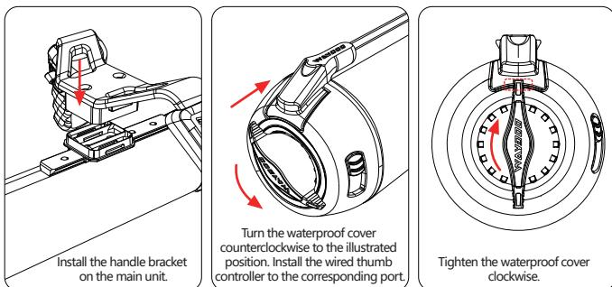
Note: Please install the wired thumb controller in a dry environment. Please dry the port before installation it is wet.
