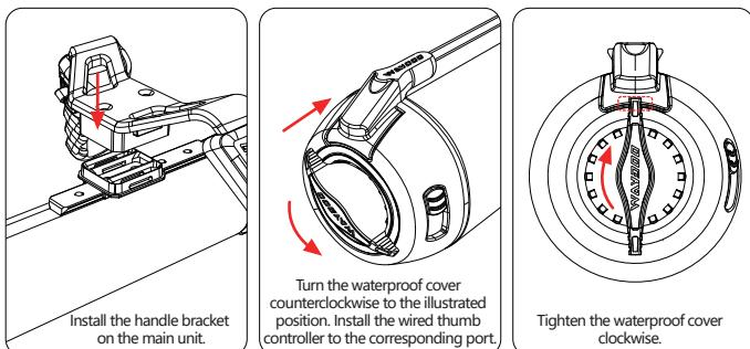
Note: Please install the wired thumb controller in a dry environment.
