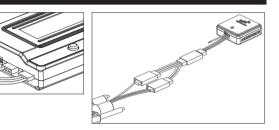
• The Seaking Pro 120A/160A ESC can also be programmed via a WiFi module along with smart phone devices (HOBBWYING WiFi LINK software needs to be installed on the smart phone). Before programming, users will need to connect the WiFi module to the ESC via a Y harness. For detailed information about ESC programming via WiFi module, please refer to the user manual of Hobbywing's WiFi Express.
