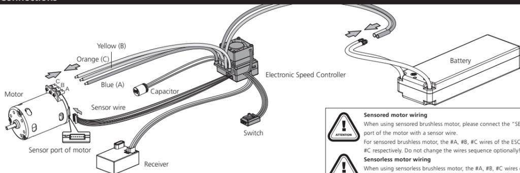
**Sensored motor wiring**
