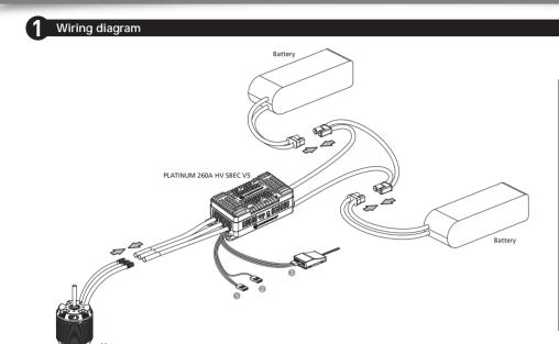
① BEC output wire (red, brown): The additional BEC output wire is plugged into the receiver battery dedicated channel or any available channel. (For better BEC power output, it is recommended to insert the BEC cable into a battery-specific channel or any available channel)
