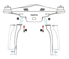
First, insert the securing pins through the holes on the highlighted diagonal position shown below. Align gimbal adapter with the four screws holes on the bottom of Phantom 2. Then align the damping unit upper plate with the gimbal adapter. Ensure both the gimbal adapter and the damping unit are aligned the gimbal adapter and the damping unit are aligned with the nose of Phantom 2. Screw the gimbal adapter and the damping unit upper plate in place.
