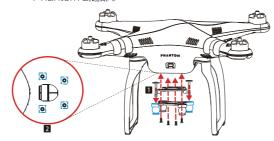
4 Attach the damping unit bottom plate to the upper plate using four vibration absorbers. Insert the securing washer firmly into correct position shown in the position shown below to secure the damping unit. Do not push too hard on the securing pins. Refer to the H4-3D Quick Start Guide for full mounting instructions.
