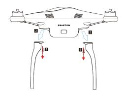
2 | Install longer landing skids (7mm longer) then reconnect cables.
